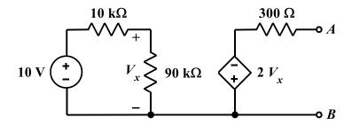
Find the Thévenin equivalent circuit with respect to terminals A and B.
